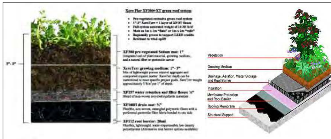
Figure 15 Example profiles : Left: Roll out system (Xeroflora.com); Right: modular tray system
