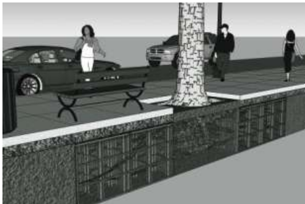
Figure 9 Silva Cells below permeable paving Copyright 2008. Casey Trees. Washington D.C.
